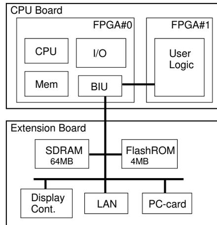
Figure 6: Mappi: the M32R FPGA evaluation board; it has the M32R softmacro on FPGA (CPU, MMU, Cache, SDI, SDRAMC, UART, Timer), FPGA Xilinx XCV2000E  $\times 2$ , SDRAM(64MB), FlashROM, 10BaseT Ethernet, Serial 2ch, PC-card slot  $\times 2$ , and Display I/F(VGA)
