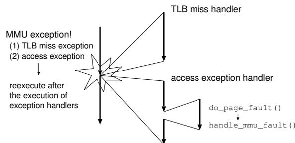
Figure 4: Exception handling for the demand-loading operation
