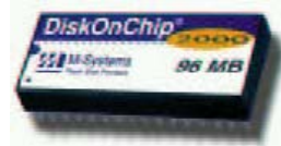
Figure 5: Le Disk On Chip de M-System
