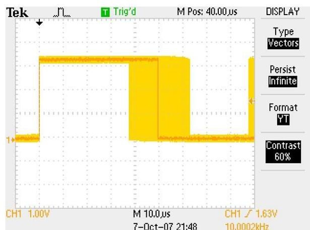
**FIGURE 24:** Jitter on LXRT (RTAI v3.5)
