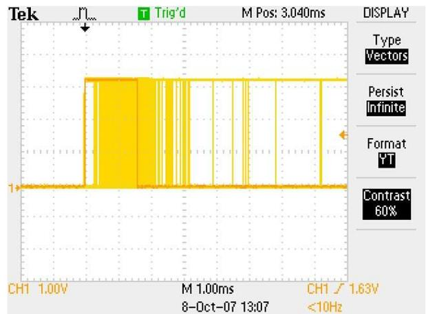
FIGURE 11: Jitter on 2.6.23-rc1 CONFIG\_PREEMPT, VIA C3 600MHz
