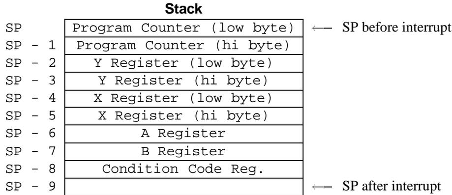
Figure 4: Diagram of Stack After an Interrupt Call
